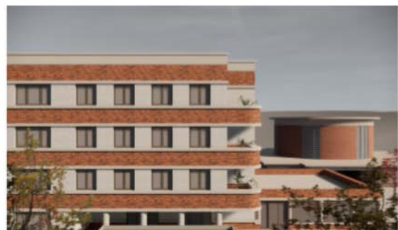
Proposed banding to head & sill - Contrasting brick
